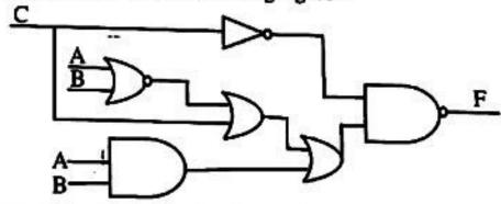
Q.5 Complete the truth table for the combinational circuit shown in the figure -
