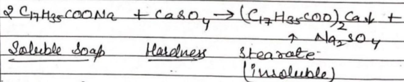
So we can determine total hardness of water by means of its titration against a standard soap solution. The appearance of lather indicates the end point of titration.
