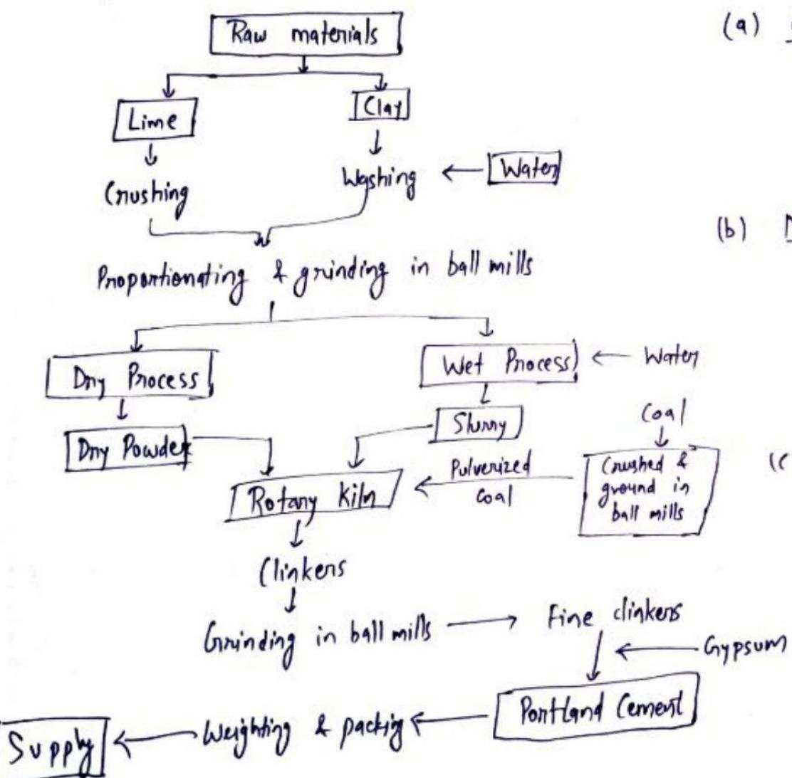
(a) Crushing:- Raw materials are grinded in ball mills & passed to tube mill conveyed through means of screw driver. The material is mixed with 30-40% water before grinding.
