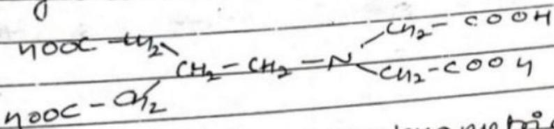
This method is complexometric titration of water sample with EDTA using Eriochrome Black T as the indicator. EDTA (ethylene diamine tetra acetic acid) is strong complexing agent.
