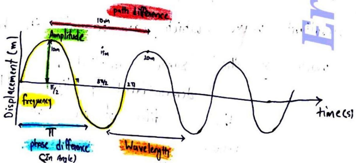
Amplitude :- maximum displacement moved by a point on a vibrating body on wave.
